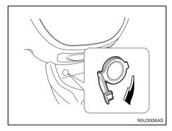
To use the outlet, remove the cover. When not in use, always cover the outlet with the protective cap. The accessory power outlet is operational when the ignition is in the ACC or ON positions.
